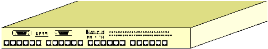
Fig 4.41 Equipment fitted with RJ45 connectors
